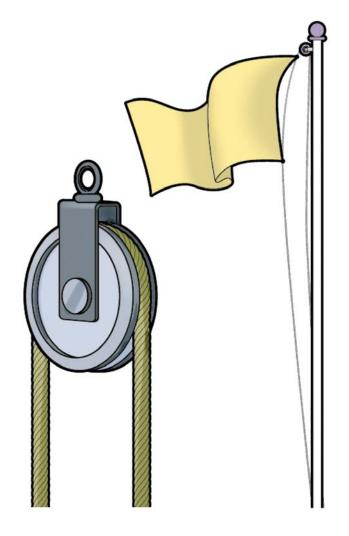
A pulley is a kind of simple machine. It makes work easier. The flagpole has a simple pulley. The pulley makes it easier to raise and lower the flag.
