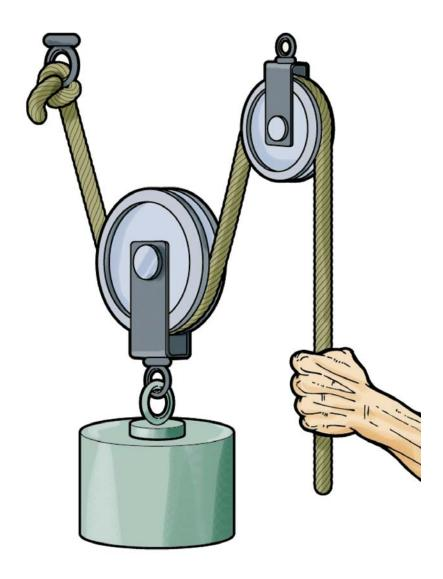
Sometimes two or more pulleys are combined. They reduce the amount of push or pull needed to do work.
