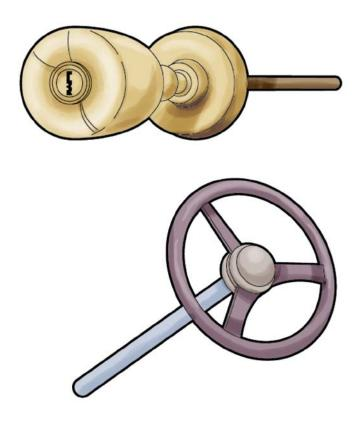
A doorknob and a steering wheel are wheels and axles. The doorknob makes it easier to open a door. The steering wheel makes it easier to turn a car.
