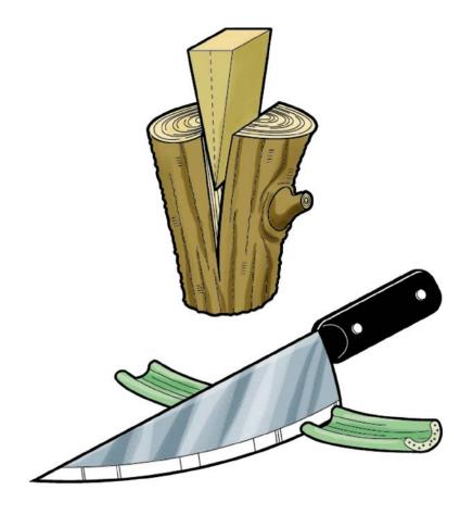
The wedge is a simple machine. It makes work much easier. It is really two back-to-back inclined planes. A knife is an example of a wedge. It makes it easier to cut things.
