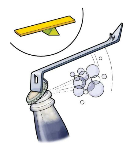
A lever is one kind of simple machine. It makes work much easier. A bottle opener is a lever. It makes it easier to open a bottle.
